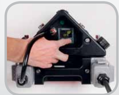
Setting temperature and pressure controller
